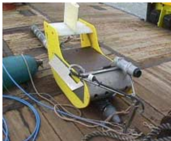
Nv-Shuttle with USBL transponder on its port bow and magnetometer underneath
